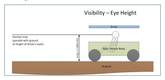
5.9.1 **Forward Visibility** - From the normal driving position, all drivers must be able to see, without artificial assistance: (1) a point on the ground 8 meters in front of the solar car.
