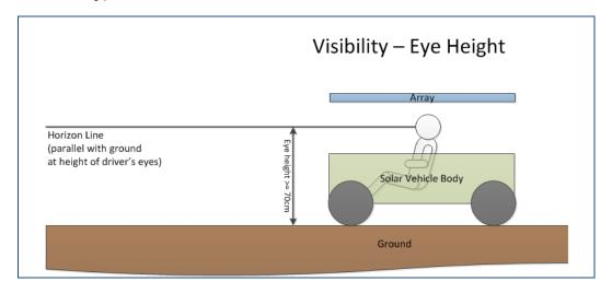
5.9.1 **Forward Visibility** - From the normal driving position, all drivers must be able to see, without artificial assistance: (1) a point on the ground 8 meters in front of the solar car.
