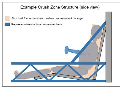
5.2.3 Roll Bar – The roll bar is the structural frame member that extends above the driver's head, protecting the driver in the event of a roll-over. The roll bar must consist of one continuous piece of metal. The bottom of the roll bar must extend at least 5 cm vertically from the top of the driver's head or helmet.
