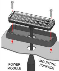
Drill a 0.625" diameter hole in the mounting surface to pass the cable through.
