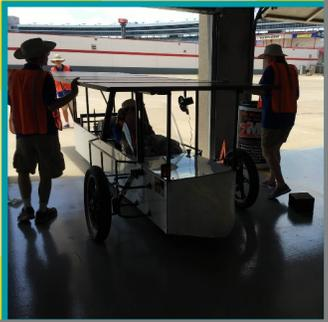
*Station 1: General Scrutineering - Documentation, Vehicle Size, Roll Cage, Roll Bar, Crush Zones, Vehicle Points, Driver Conditions, & Student Involvement.*
