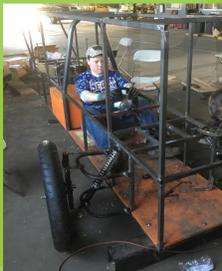
*Jake is adding the steering wheel and testing out the steering system. We have ability to turn the wheels!*
