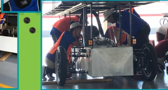
*Mark worked nearly all night long, completely re-engineering and rebuilding the motor mount assembly to be able to handle the high torque loads associated with the electric motor. This was finally the silver bullet that solved most of our nagging chain problems, which had plagued us all through the first several days of scrutineering!*
